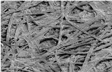
350 × 224 - Scanning electron micrograph of the surface of normal office paper. Note the various void areas between the fibers, which need to be filled in order to provide consistent print reproduction.
