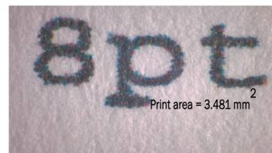
*By adjusting the surface treatment formula, Finch Paper tailored a sheet to meet specific dot gain requirements for a transactional printer using a dye-based ink system.*
